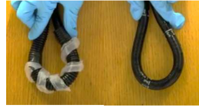
Fig. 11. Comparison of minimum bending radius between endoscope with CMES (left) and without CMES (right, positive control).
